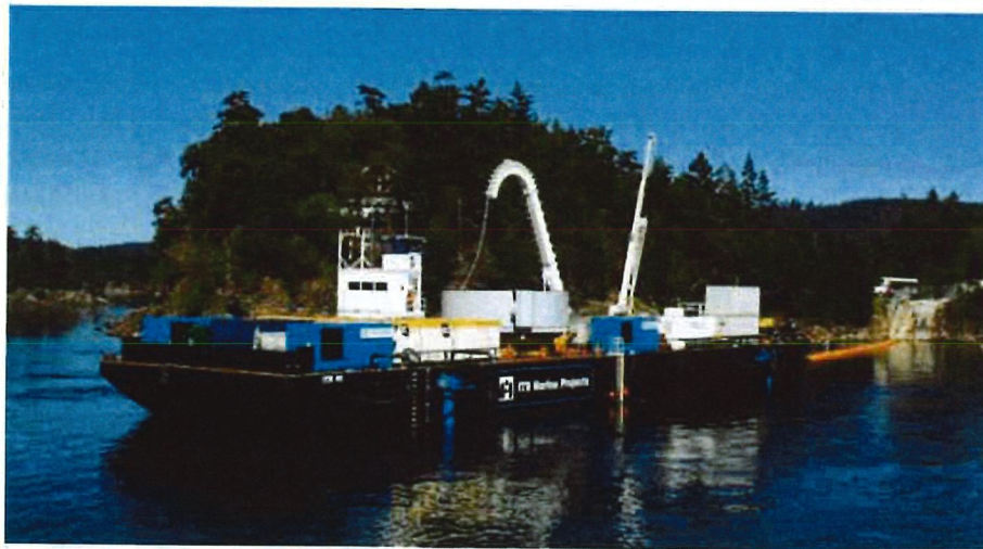
Figure 2. Standard cable laying ship and cable being deployed as ship departs landing.
